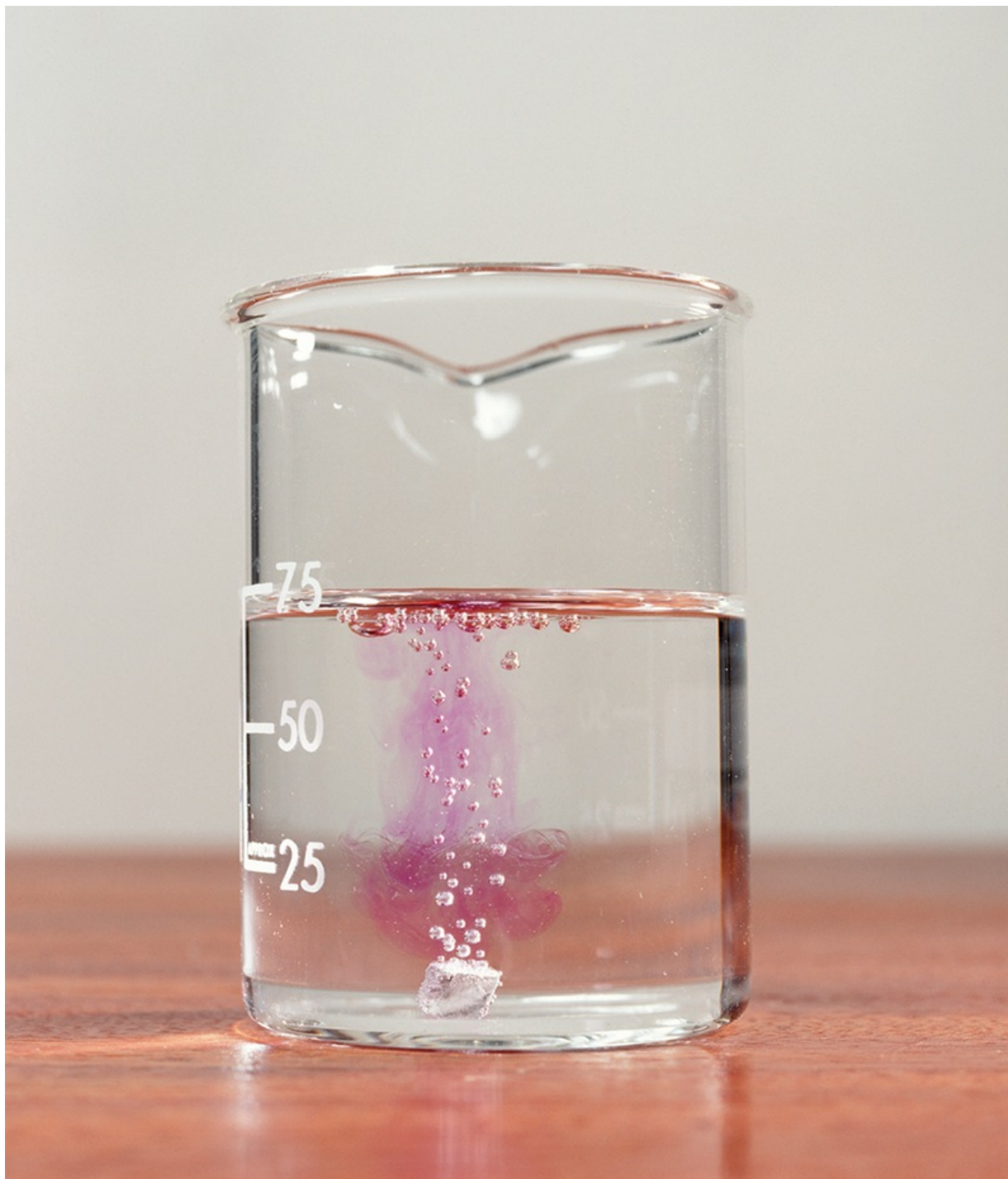
Figure 17.5: Sodium reacting with ethanol. The pink colour is from a colourless phenolphthalein indicator that has been added to the ethanol, showing the basic nature of the sodium ethoxide formed in the ethanol.
