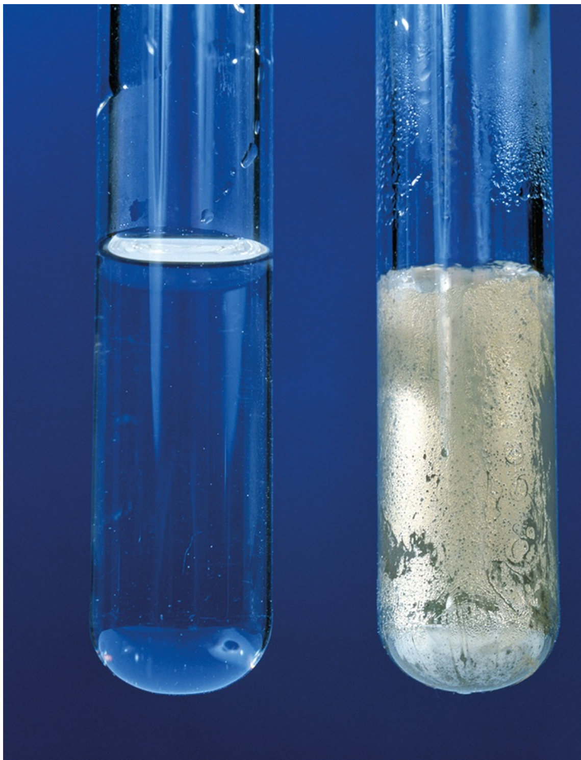
Figure 18.4: The 'before' and 'after' observations when Tollens' reagent is warmed with an aldehyde, such as ethanal, \text{CH}_3\text{CHO} .
