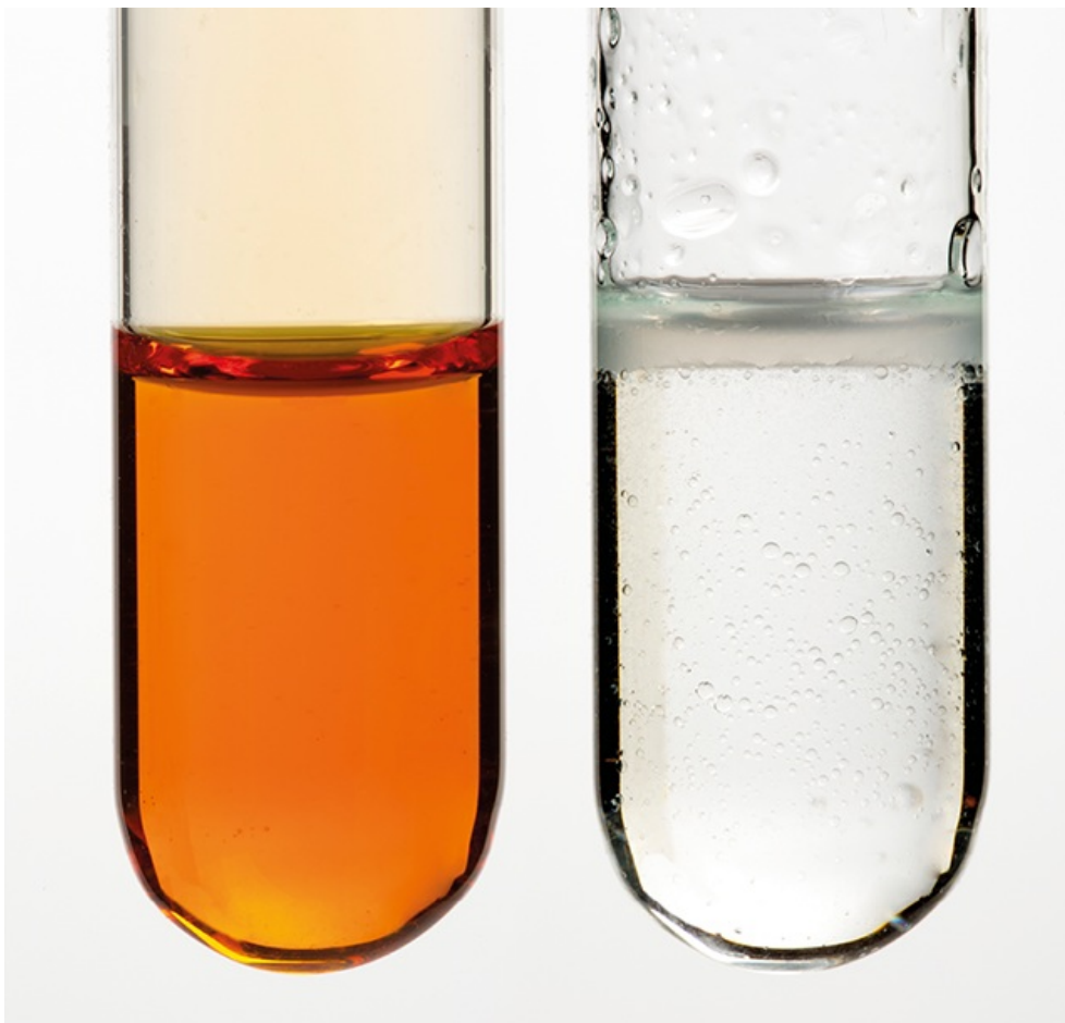
Figure 15.17: The addition reaction used to test for an unsaturated compound.
