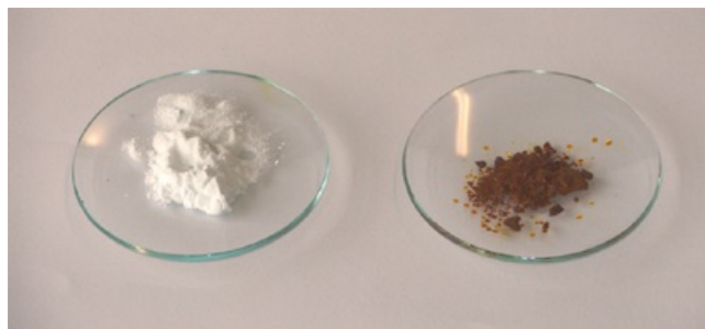
Figure 3.18: Iron(II) chloride (left) and iron(III) chloride (right). These two chlorides of iron both contain iron and chlorine, but they have different formulae.
