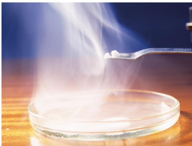
Figure 10.14: Solid phosphorus(V) chloride is hydrolysed in water, releasing white fumes of hydrogen chloride gas.
