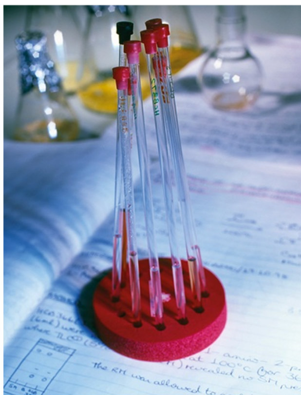
Figure 30.17: Samples dissolved in a solvent in narrow tubes ready for NMR analysis.
