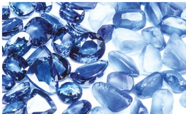
Figure 5.8: Sapphires sparkle in the light when polished. They are cut by exerting a force on the cleavage planes between layers of ions in the crystal.
