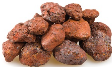
Figure 3.16: This iron ore is impure \text{Fe}_2\text{O}_3 . We can calculate the mass of iron that can be obtained from \text{Fe}_2\text{O}_3 by using molar masses.
