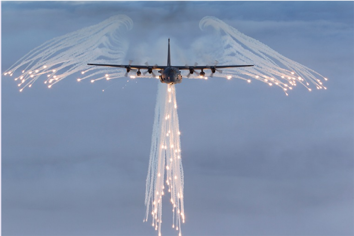
Figure 11.1: A military plane releasing its decoy flares to protect itself from missile attack.
