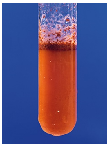
Figure 27.8: The azo dye (also called a diazonium dye) forms in a coupling reaction between the diazonium ion and an alkaline solution of phenol.
