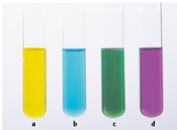
Figure 24.2: Vanadium and its oxidation states: a a solution containing \text{VO}_2^+ ions, b a solution containing \text{VO}^{2+} ions, c a solution containing \text{V}^{3+} ions, d a solution containing \text{V}^{2+} ions.
